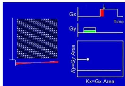
**Figure 30.** Creating stripe patterns in arbitrary directions with the sequential application of  $G_y$  and  $G_x$  gradients. A K-space plot traces out the area of the  $G_x$  and  $G_y$  gradient for the  $K_x$  and  $K_y$  locations respectively.
